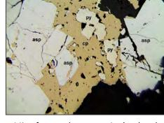
Microfractured arsenopyrite (asp) and pyrite (py) surrounded by chalcopyrite (cp). Sample **DD-2 703'**.
