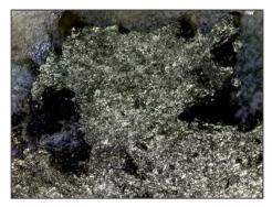
DD - 2 654 ft Chalcopyrite in siderite
