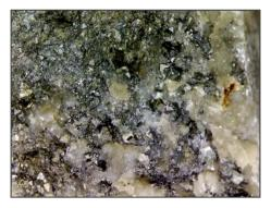
**DD – 2 701 ft** Arsenopyrite-tetrahedritechalcopyrite in siderite
